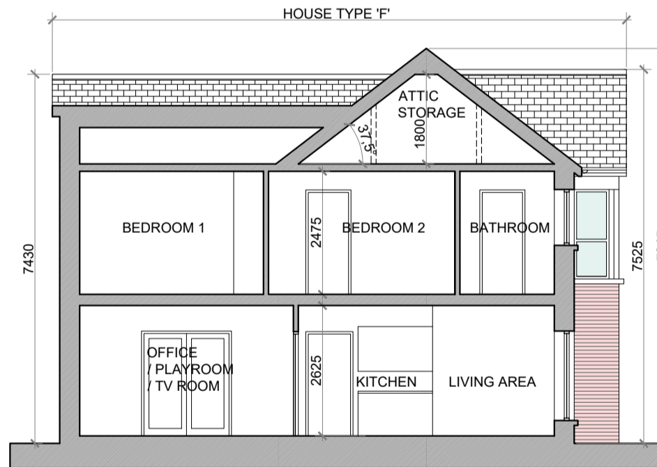
SECTION A-A @ 1:100 TERRACE BLOCK TYPE 16
